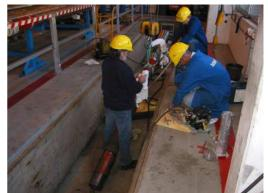
The set up of the test was a 7" communication nipple where we made a longitude damage on the lower seal area. We thereafter ran a 7" insert valve with V-packing into the nipple. A 760 meter control line was connected and flushed through with hydraulic oil. The damage on the sealing area was that big that we could not open the insert valve.
